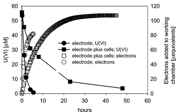
**FIGURE 2.** Uranium removal and corresponding electron balance using a poised graphite electrode ( $-500$  mV) with and without *G. sulfurreducens*. Filled and open data markers correspond to the uranium concentration and the cumulative electrons added to the working chamber, respectively, under each condition.
