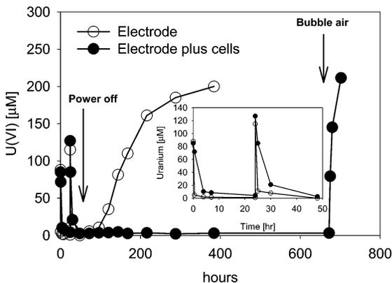
**FIGURE 1.** Uranium removal and recovery in the presence of a potentiostat-poised graphite electrode in the presence and absence of *G. sulfurreducens*. The potentiostat was poised at  $-500$  mV (vs a Ag/AgCl reference). The inset figure shows a shortened time axis for the same data set which better illustrates the addition and removal of U(VI). Uranium was added at  $t = 0$  h ( $80 \mu\text{M}$ ) and  $t = 24$  h ( $120 \mu\text{M}$ ).
