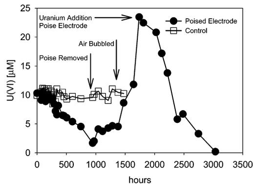
**FIGURE 3.** Removal and recovery of U(VI) in batch incubations of uranium-contaminated soil and groundwater from Rifle, CO. After 96 h, the initial poise was set at  $-500$  mV (vs Ag/AgCl). It was adjusted to  $-600$  mV at 170 h and  $-700$  mV at 314 h. Power was turned off at 970 h, and air was bubbled into the system at 1474 h. At 1738 h, more U(VI) was added and power was reapplied at a potential of  $-700$  mV.
