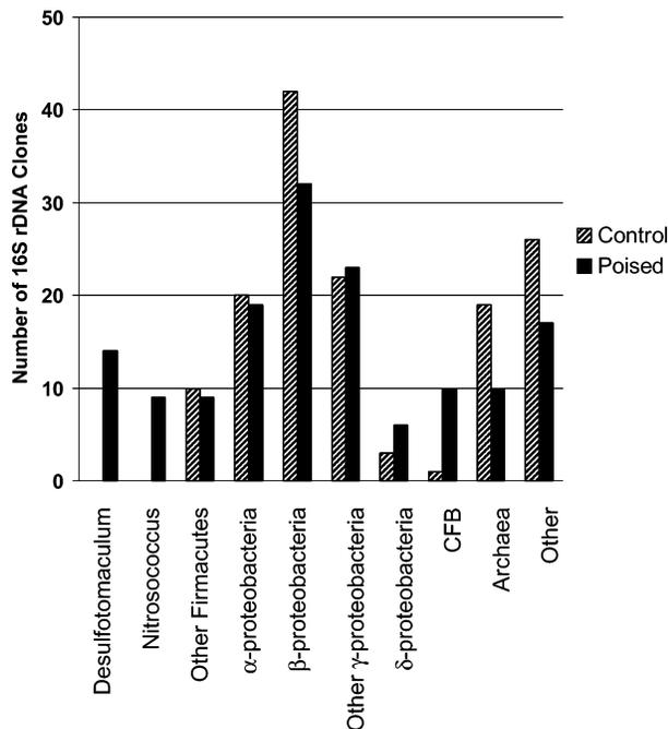
**FIGURE 4. Comparison of 16S rRNA clones found on poised and unpoised (control) electrodes during remediation of uranium contamination of soil and groundwater. A total of 144 clones from each sample were analyzed. Clones were placed into groups based on the closest percent similarity in the database as determined by the BLASTn algorithm (41).**
