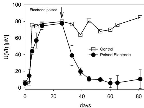
**FIGURE 5. Uranium removal by graphite electrodes in flow-through columns packed with uranium-contaminated soil from Rifle, CO. Columns were fed with uranium-containing groundwater from Rifle, CO. The working electrodes in the control column were not given a poised potential. Samples were removed from the 11 cm sampling port. The results represent the mean and range of the results from two columns.**
