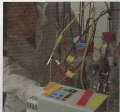
University of Massachusetts-Amherst postdoctoral associate Hana Yi takes a reading from a microbial fuel cell.
