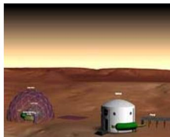
Conceptual drawing of a Mars base based on bio-power. A greenhouse, microbial fuel cells, and algal growing compartments are all visible. Image by Chris Lund. Credit: IntAct Labs
