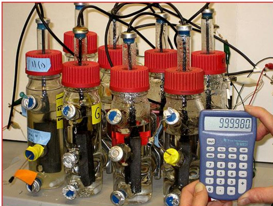
Bacteria in these flasks are making enough current to run this calculator. Courtesy [Geobacter Project](#)
