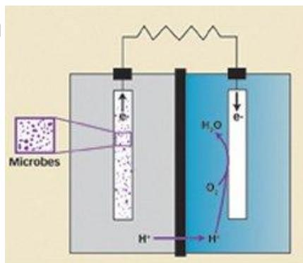
**POWER BASICS.** *Microbes on the anode (in left chamber) deposit electrons (e<sup>-</sup>), which travel along a wire to the cathode (in right chamber). Protons (H<sup>+</sup>) move through a selective membrane from anode's chamber to cathode's chamber, where they combine with electrons and oxygen to form water.*
